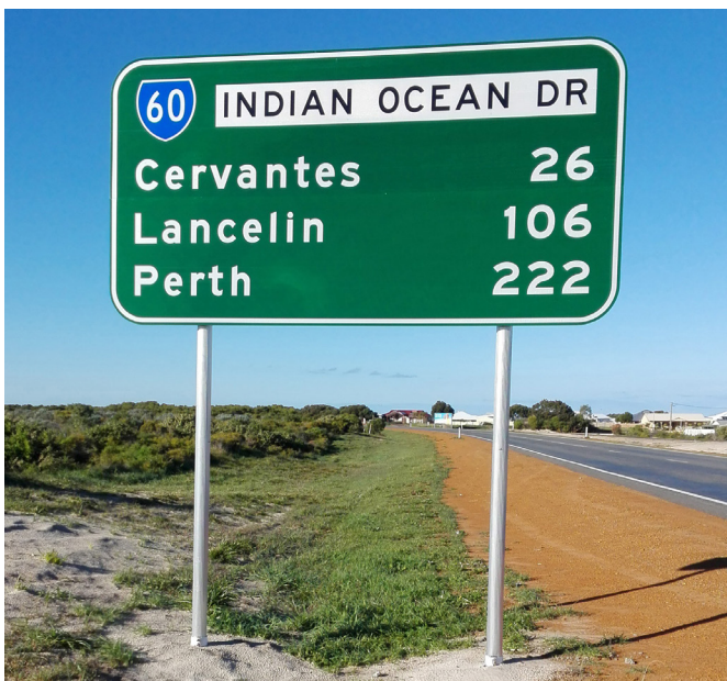
Signfix frangible poles range 60-114mm in outer diameter and hold up to 16m 2 road signs in Australian wind regions.
